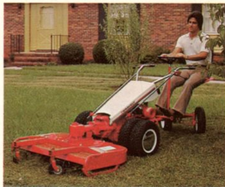
Gravely 8 hp Convertible Tractor, with 40" Twin-Blade Rotary Mower with optional Steering Sulky and dual wheels.
